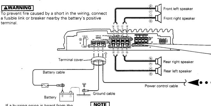
If a buzzing noise is heard from the speakers when the engine is running, connect a line noise filter (optional) to each of the battery cable.
