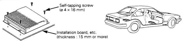
Since the power amplifier has no parts which require operation, it can be installed at a position away from the driver's seat without any hindrances.
